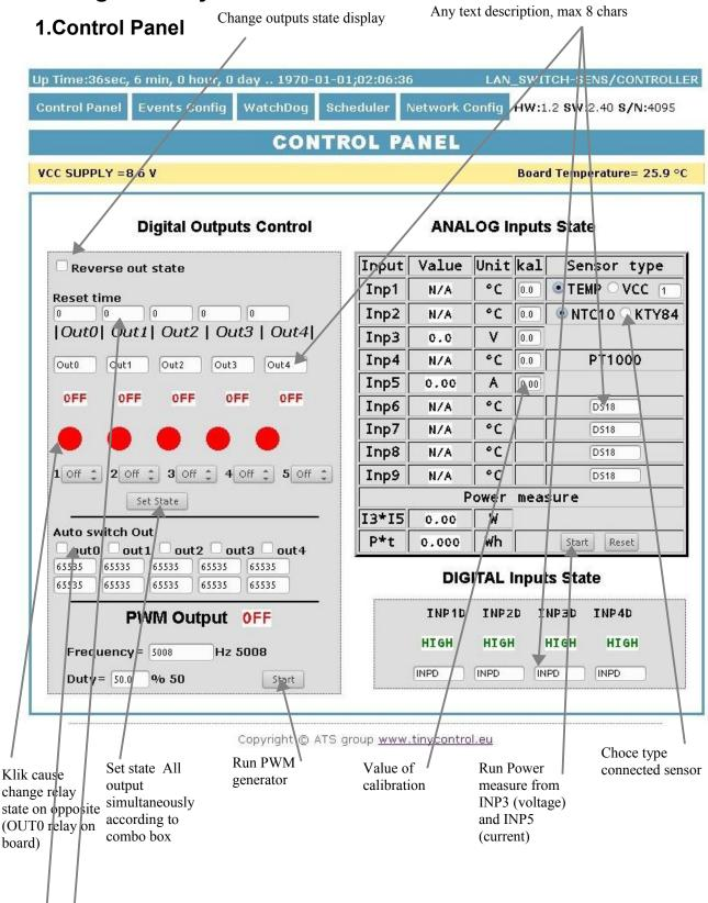
**Reset time** – for 0 normal outputs work (ON/OFF), for time > 0 output after push button change state and return to state before after the specified time in seconds (max 65534).
